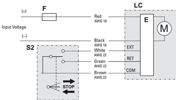
The direction of the extension tube travel is controlled by switching the COM (common) output to the EXT (extend) or RET (retract) inputs.
