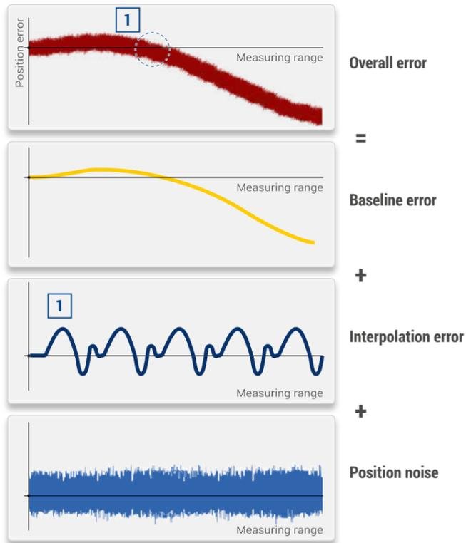
The accuracy of a linear encoder is mainly determined by the baseline error of the graduation carrier, the interpolation error of the optoelectronic scanning and the position noise.
