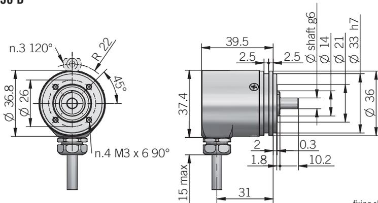
recommended mating shaft tolerance H7
