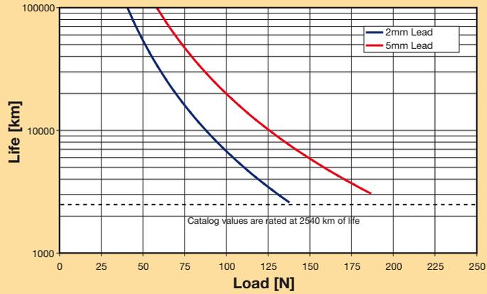
**403XE Ballscrew Life with Axial Load**
