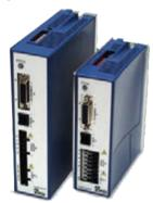
Full Featured AC or DC Input Stepper Drives with Intelligent Indexing Option (-PN)
