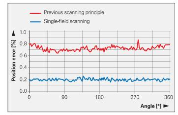
Position error within one signal period (example: RCN 2580, 1% position deviation  $\triangleq$  0.8")
