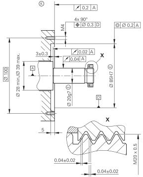
mm  $\Box$ Tolerancing ISO 8015 ISO 2768 - m H < 6 mm: ±0.2 mm
