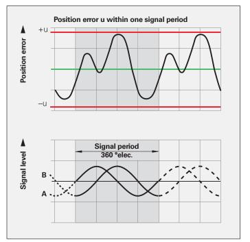
For its angle encoders with integral bearings, HEIDENHAIN prepares individual quality inspection certificates and ships them with the encoder. The quality inspection certificate documents the encoder's accuracy and serves as a traceability record to a calibration standard.
